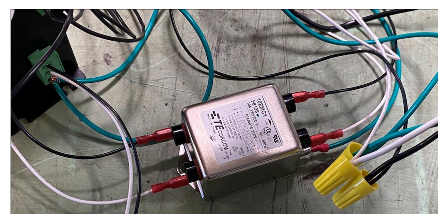
Figure 8: EMC and power cord wiring
