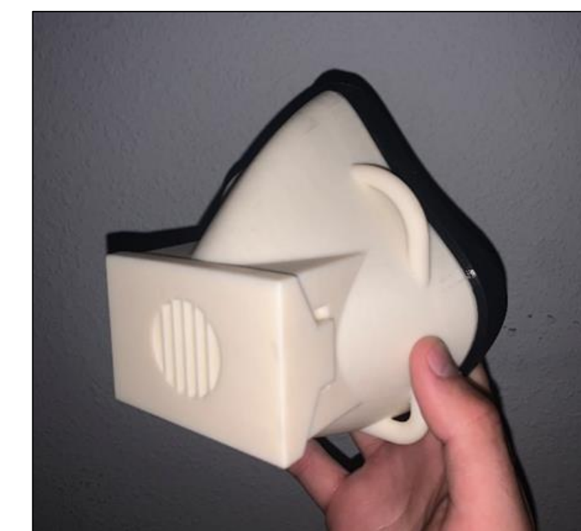
Figure 10: Final Design #1 3D Printed w/seal
