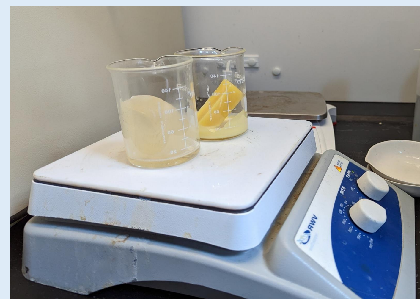
Figure 1: Preparation of wax mixtures (glycerin and beeswax)
