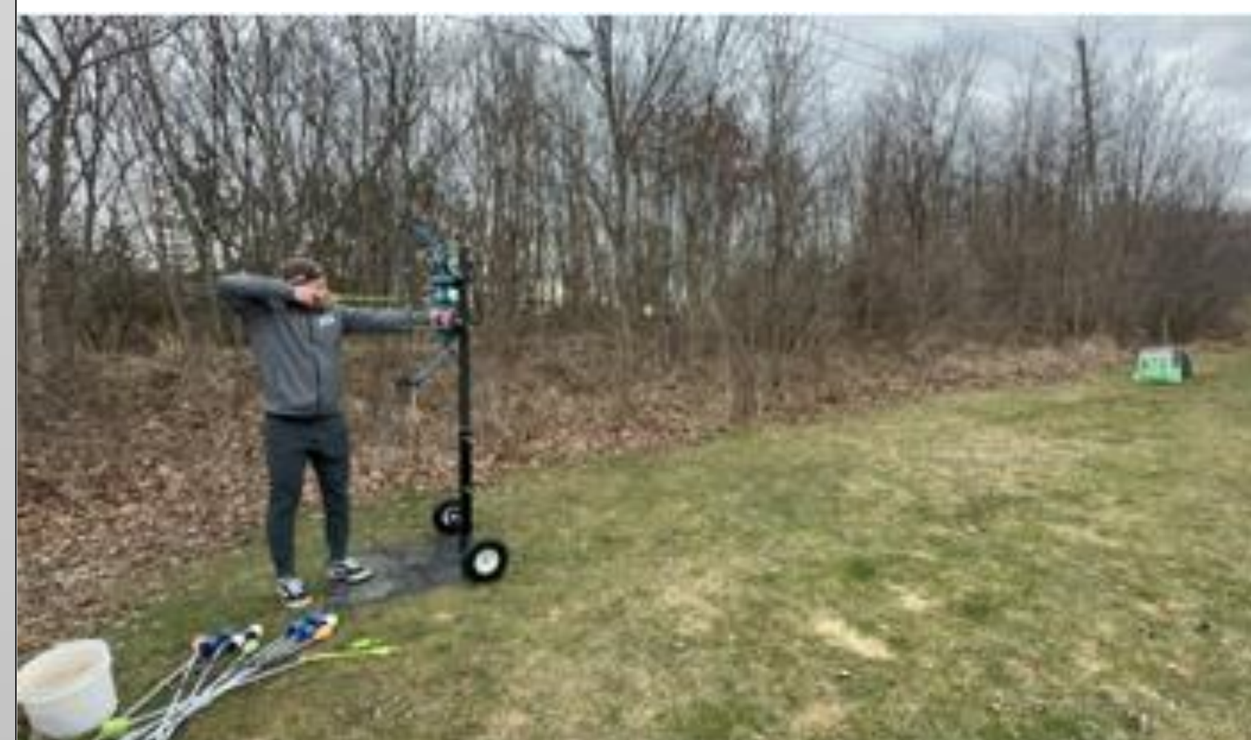
Archery Range Testing: Validate that the device could mimic any conditions experienced without losses in overall accuracy
