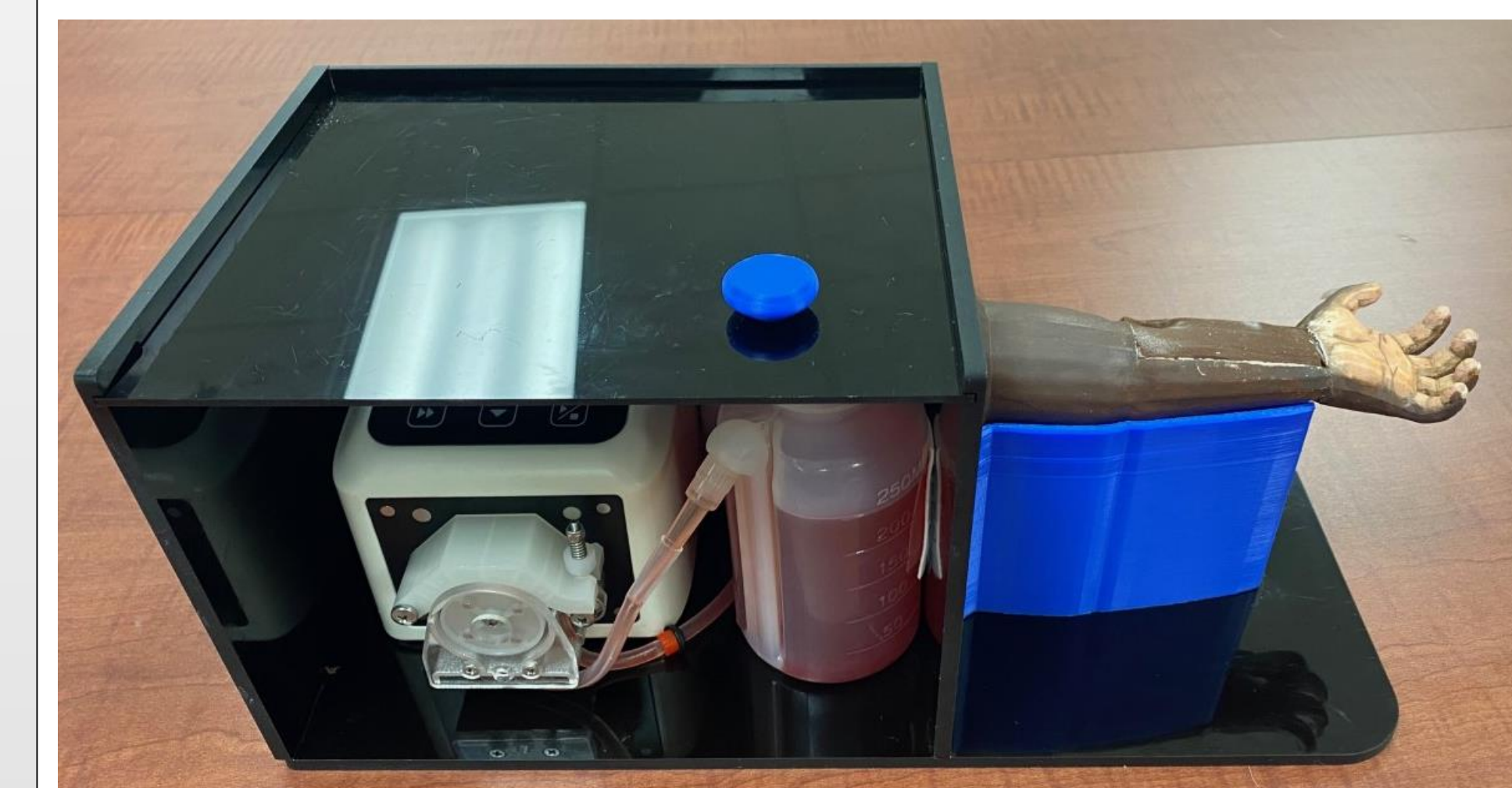
Figure 17 : Final Design of Neonatal ABG Trainer
