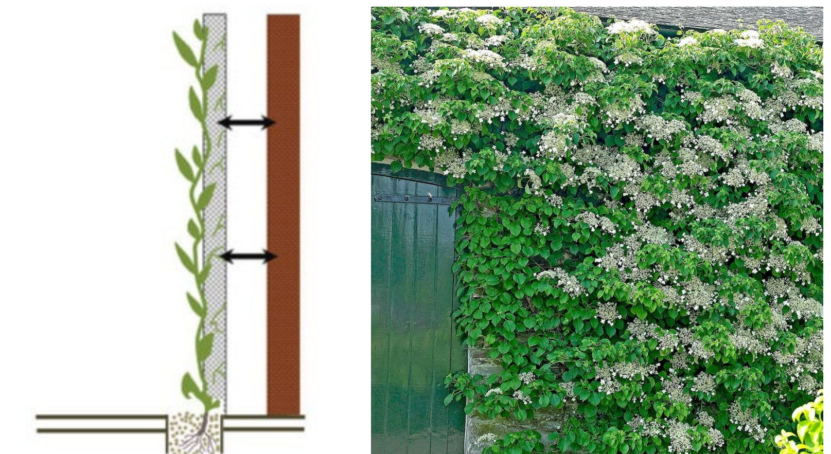
Figure 6: Type II Extensive Green Wall
