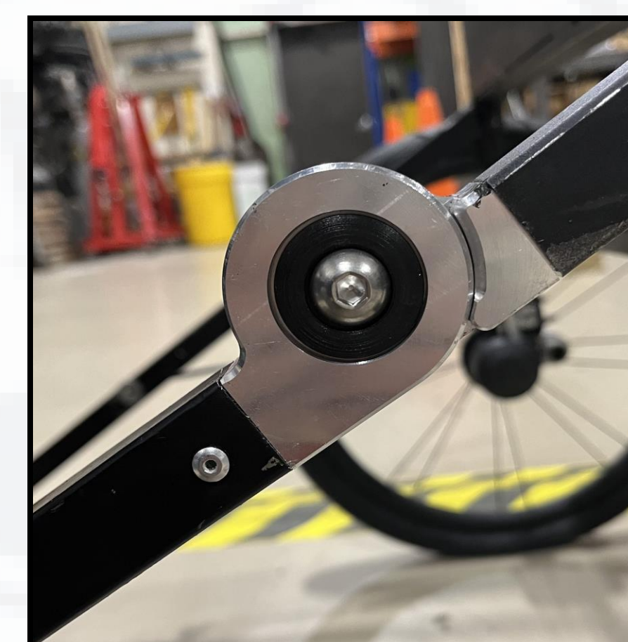
Image 6: CNC machined hinges
