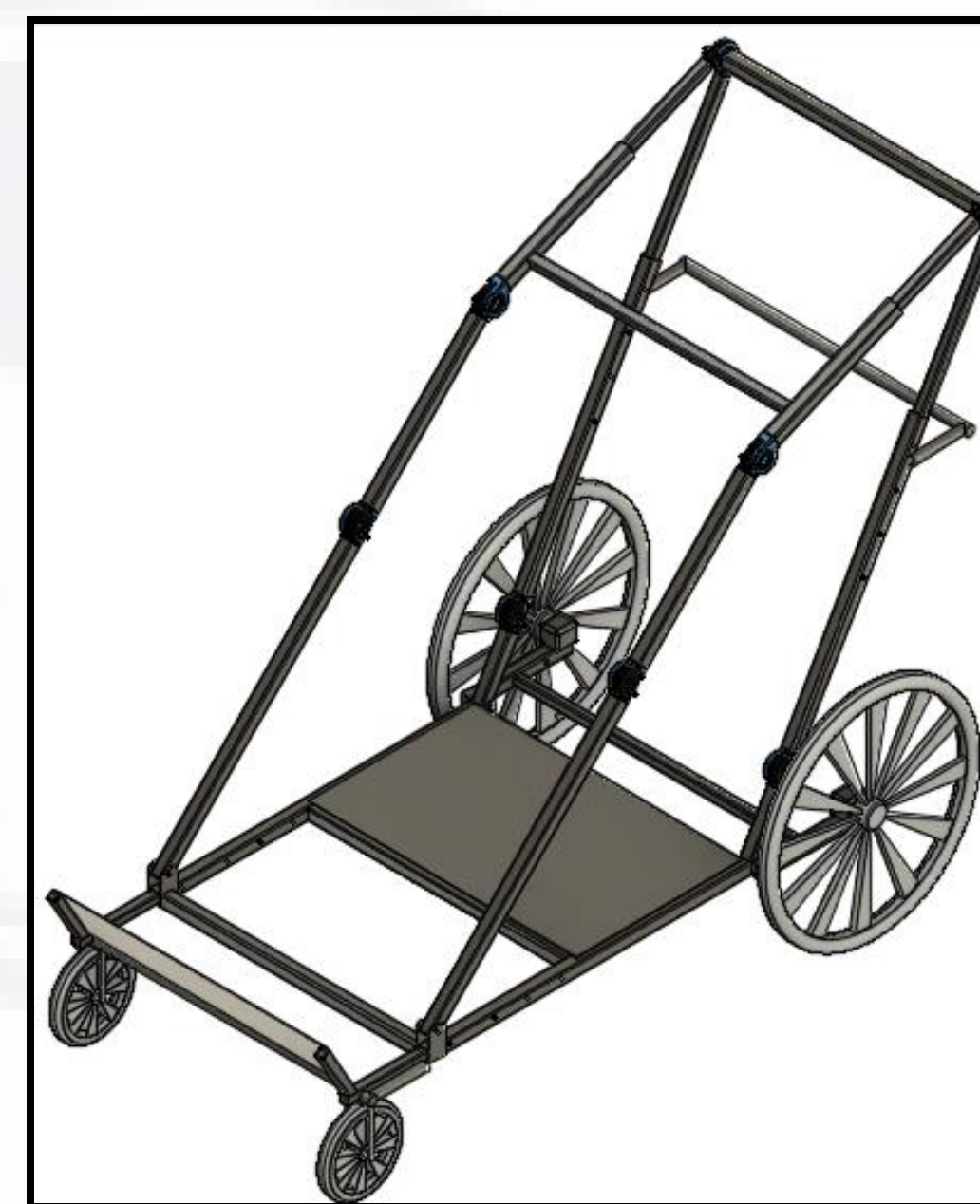
Image 3: SolidWorks™ 3D model of stroller
