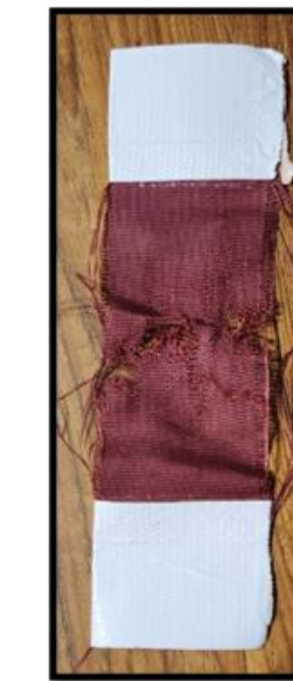
Image 7: Fabric specimen post-Instron yield test
