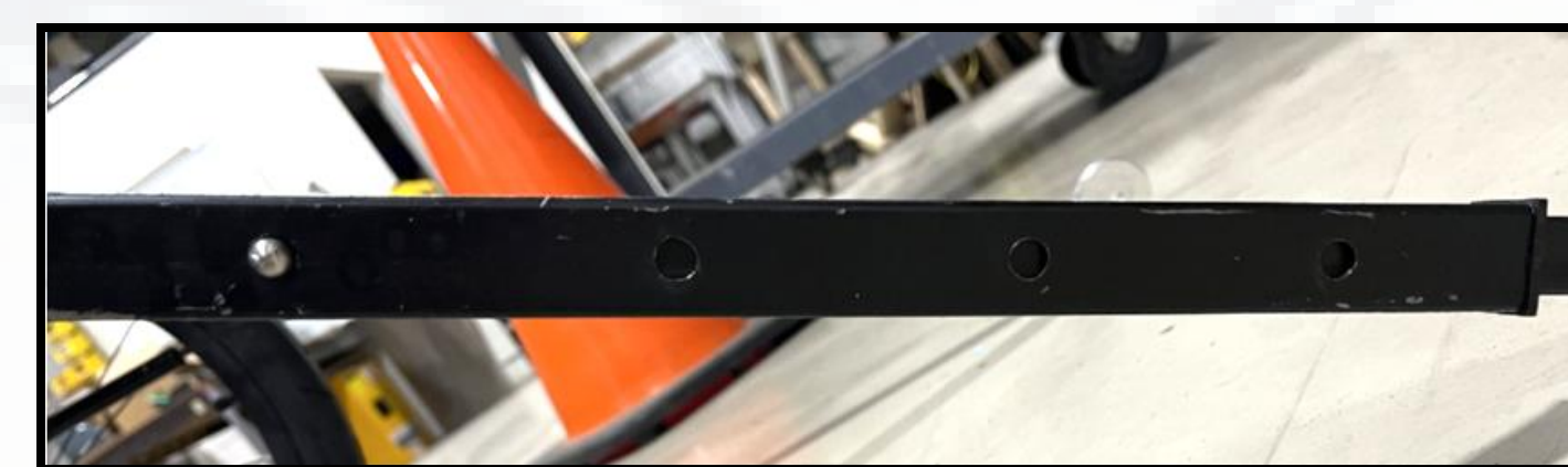
Image 5: Push button system of telescoping elements
