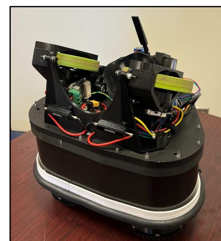
Figure 4. Assembled Quarterback Mechanism
