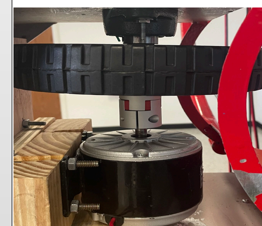
Figure 6: Wheel, Shaft, Coupling and Bearing
