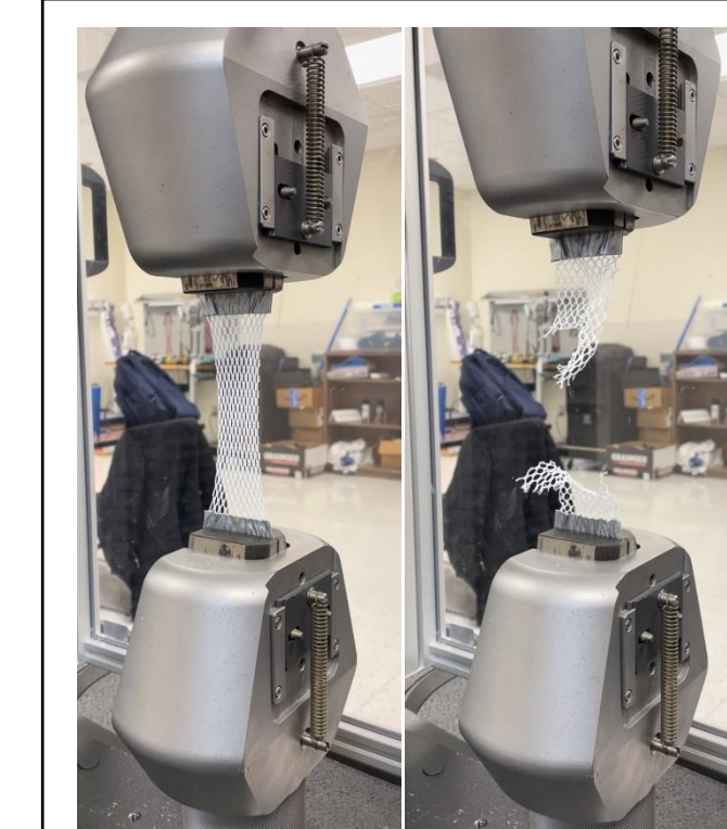
Figure 12. Tensile Testing Setup
