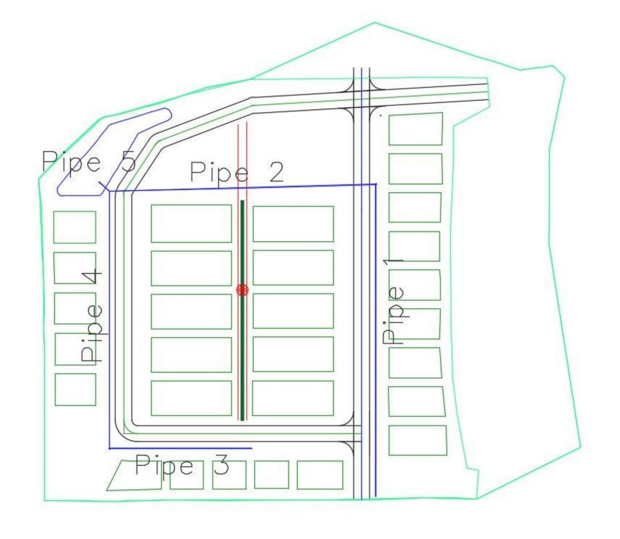
Our Project area consisted of 3 different delineated areas, one in the East, one in the South, and one in the West. We did not include a delineated area in the North end due to that water flowing into the Northern subdivision's inlets. Each delineated area contains 2 inlets for stormwater to make a total of 6 inlets.
