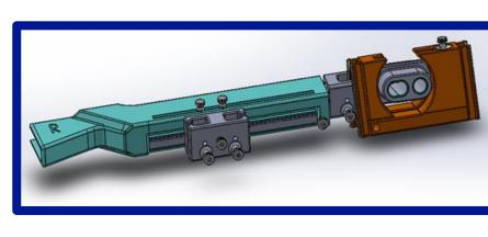
The third prototype and final design improves the prototype by increasing the length of the sliding block and moving away from geardriven mechanisms in favor of tightening bolts for easier user interface. This design is reversible, compatible with left and right leg orientations, is dynamically adjustable for all nail lengths between 220 to 500 millimeters using the three block positions and is user friendly only requiring a few adjustments prior to surgery.
