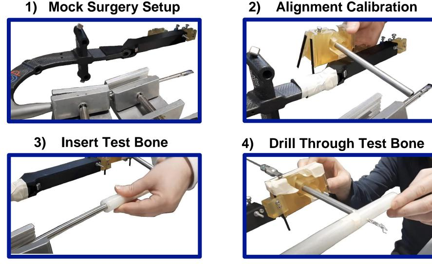
Drilling speed was measured from the moment the drill bit entered the drill sleeve to when the bit breached the opposite end of the test bone.
