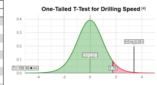
Statistical analysis showed a significant reduction in drilling speed compared to the average freehand speed of 240 seconds. The distal targeting system reduced drilling time by approximately 86%, indicating the device can successfully reduce distal locking time during surgery.
