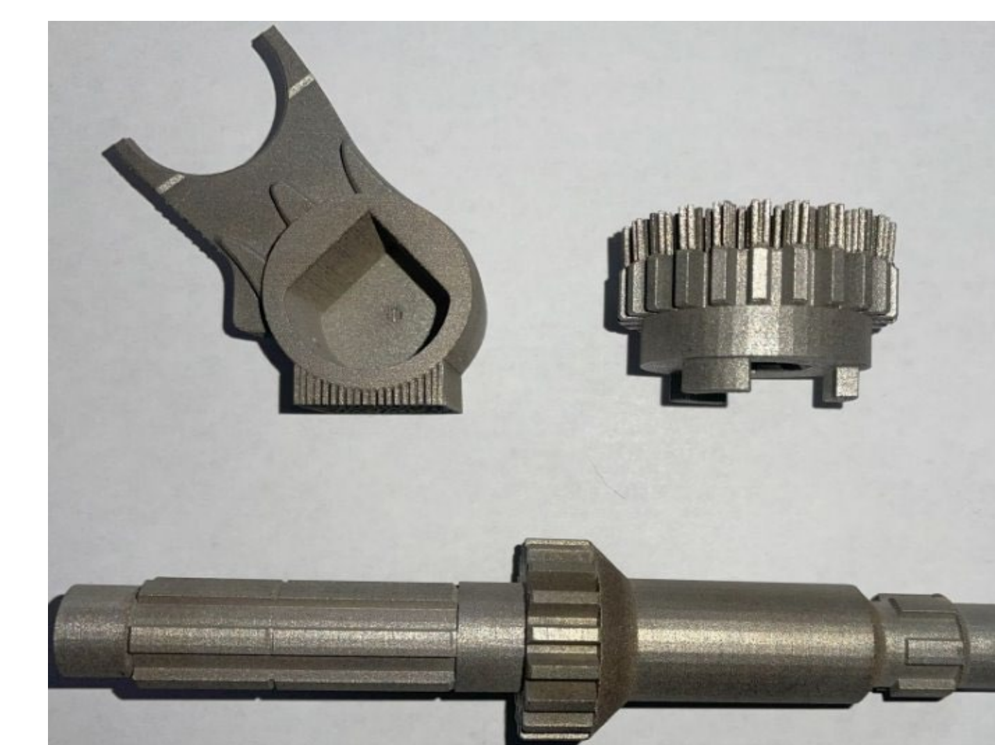
Figure 7: Metal 3D printed shaft, dog gear, and shifter fork
