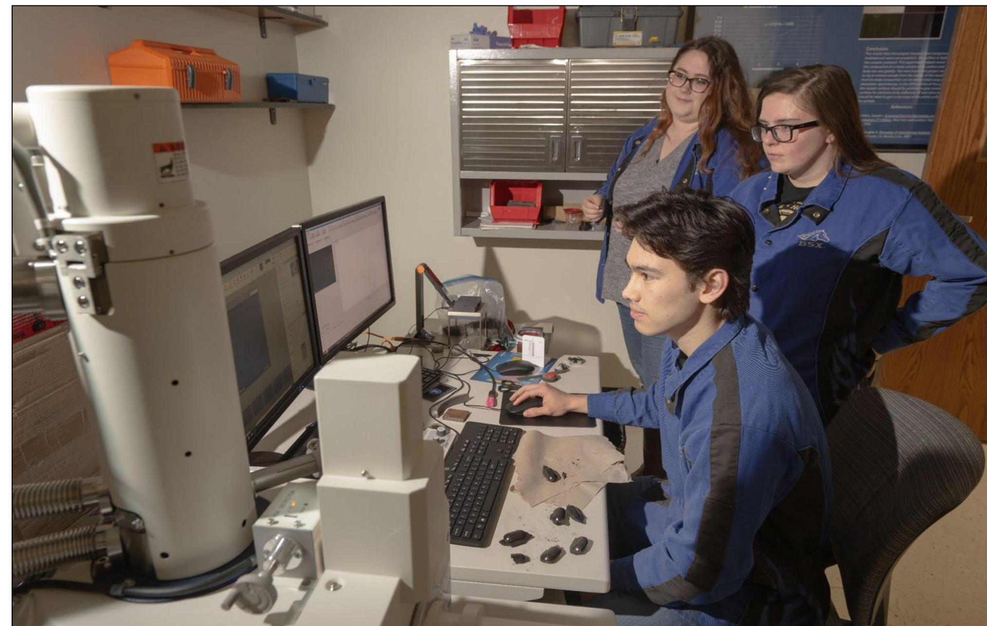
Performing a microstructure uniformity test using a Scanning Electron Microscope
