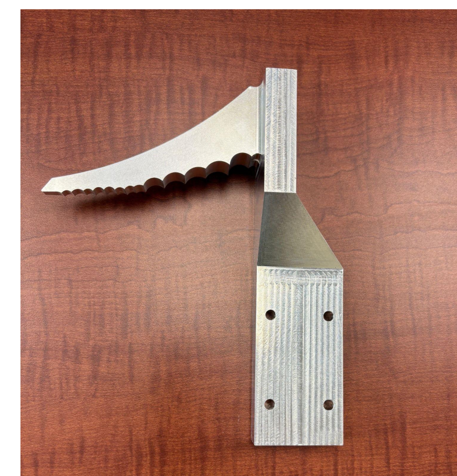
Figure 7: 6065-T6 aluminum axe head produced by CNC machine operations.
