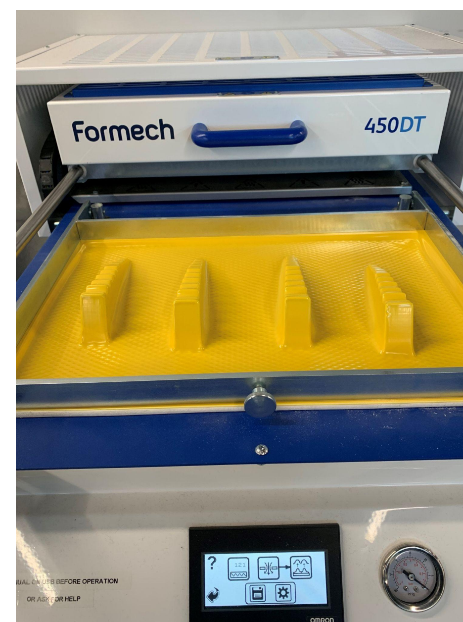
Figure 8: HIPS axe head covers produced by vacuumform.
