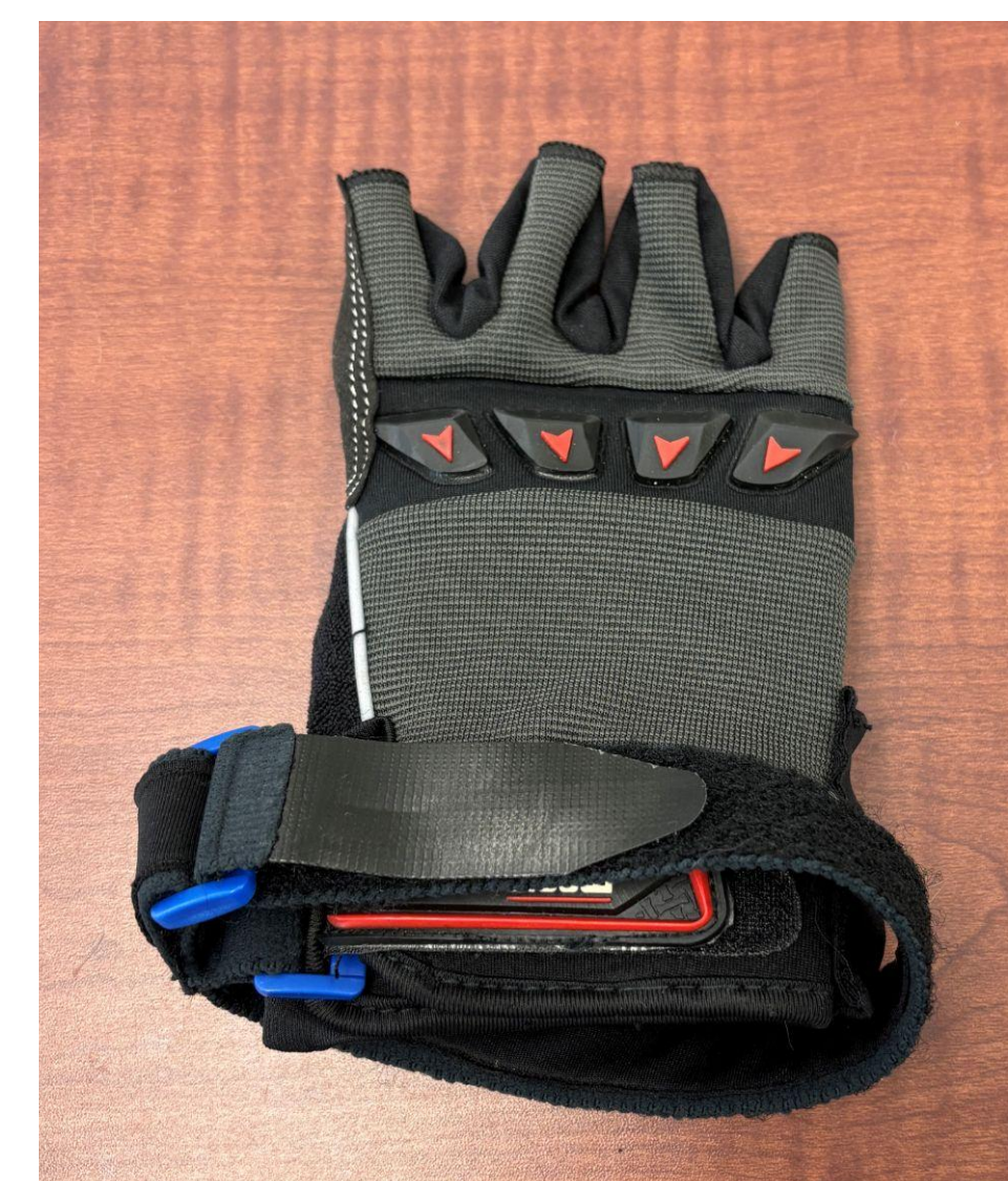
Figure 9: Safety strap made out of a glove, silicone, fabric, and a Velcro strap.
