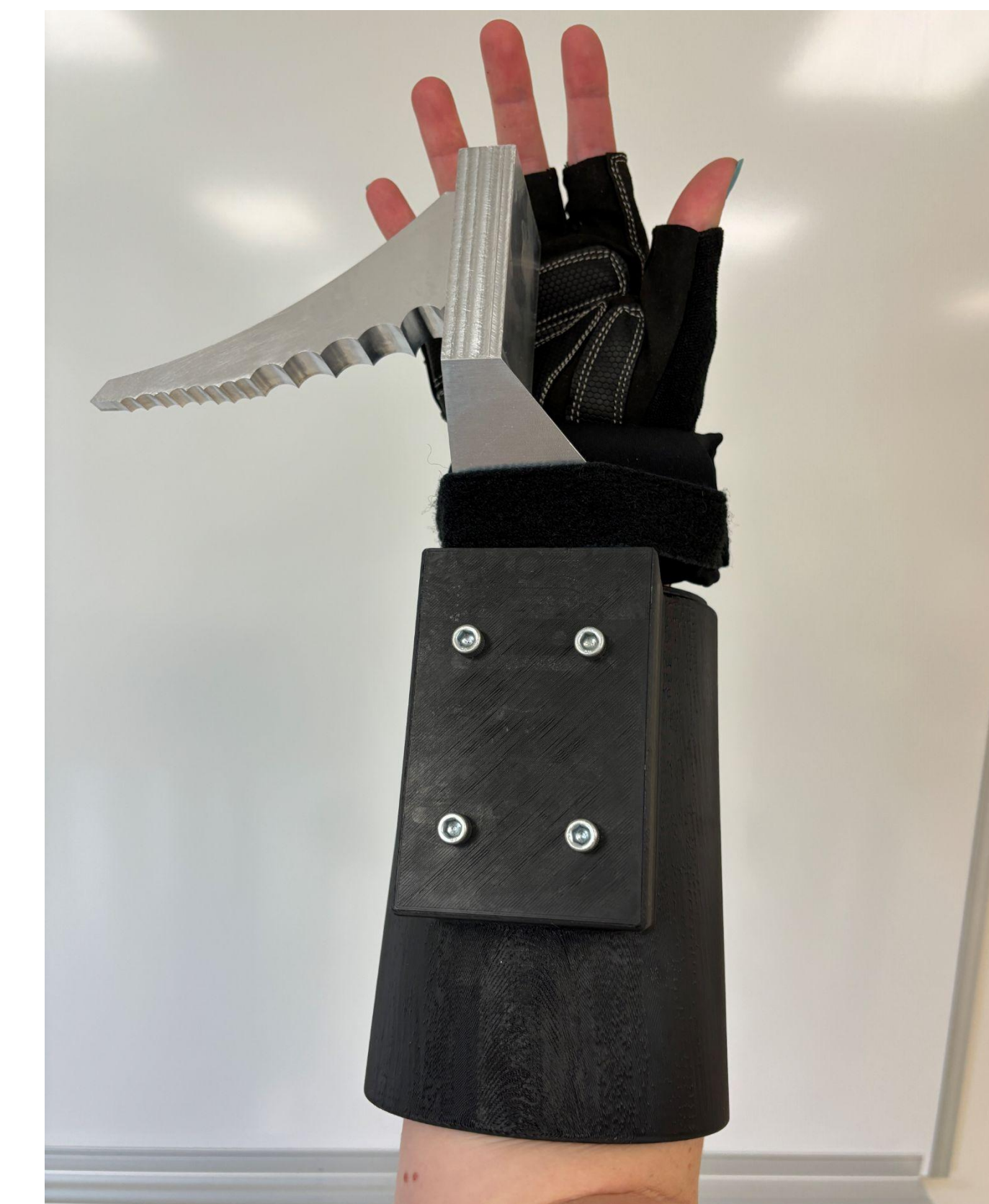
Figure 11: Final device assembly. Includes wrist/safety strap, forearm component, and axe head. Axe head covers not shown.
