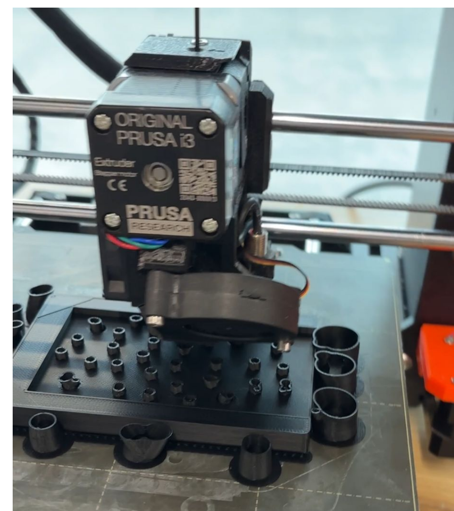
Figure 6: Forearm piece produced with PLA+ using a Prusa i3 MK3S+ 3D printer.
