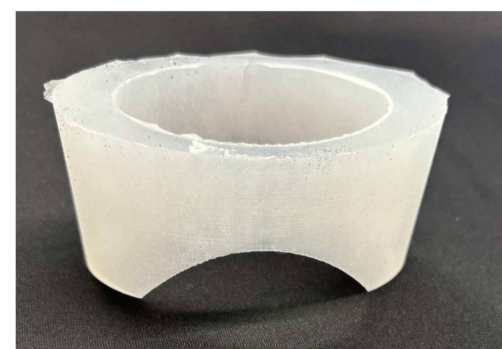
Figure 10: Device liner made out of silicone and fabric. This lies inside the forearm piece at the wrist to fill the space around the wrist.
